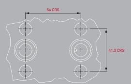
Direct Mount Instrument Connection Detail A-A
