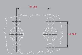
Direct Mount Instrument Connection Detail A-A
