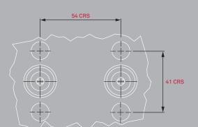
Direct Mount Instrument Connection Detail A-A
